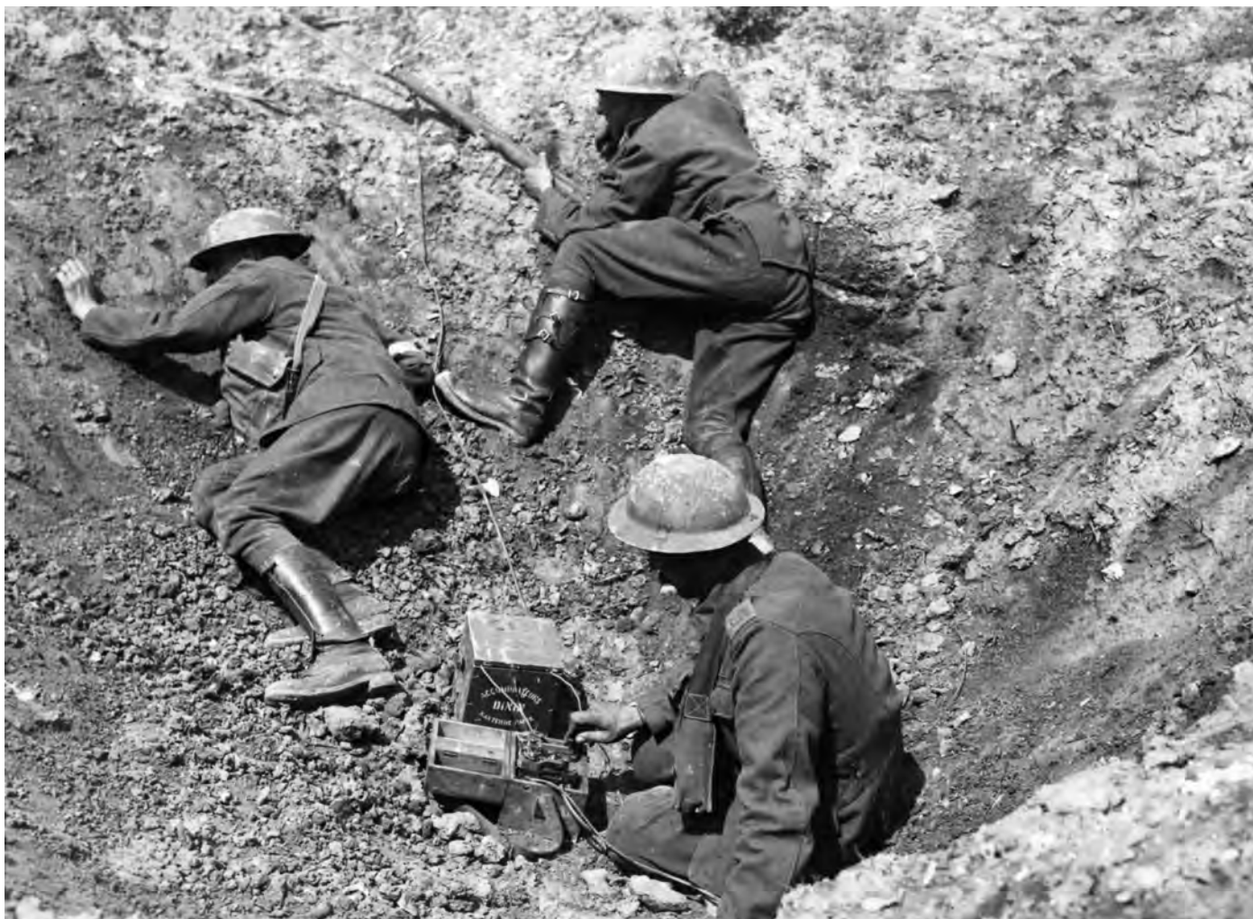
The power buzzer being operated on the front line. Note the French “Accumulateurs” battery pack.
