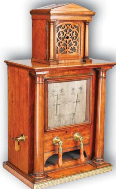
Cooke and Wheatstone Double Needle Telegraph 1844.
