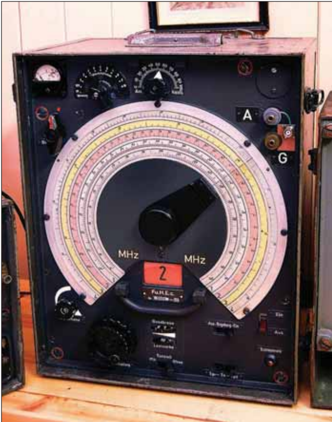
Fig 2. Intercept receiver - external view
