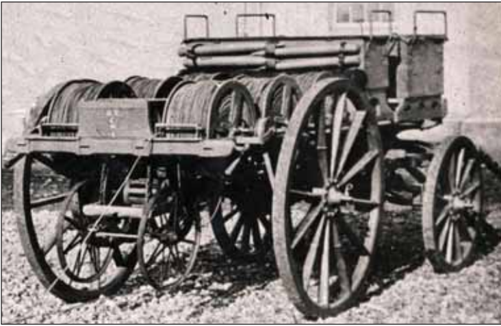
The "C" Troop Cable Wagon. The pulley attached to the "hind wheel" for reeling in the cable is visible.
